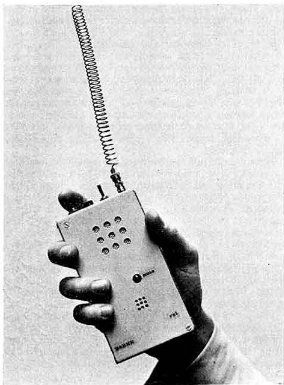
Photo 1. The 145MHz helical aerial in position on the pocket radio for which it was designed. Two-way communication at a range of 150 miles has been achieved using the combination as shown
